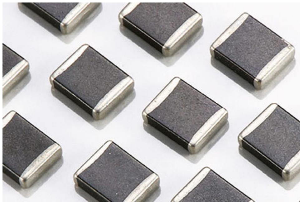
Features: small size, suitable for high density surface mount. Glass glaze coating protection, high precision, small resistance drift. Excellent weldability and solderability, suitable for wave soldering and reflow soldering. Application: rechargeable battery and temperature detection of CPU. Temperature compensation for IC, LCD and quartz oscillator. Various circuits that require temperature compensation and detection.
