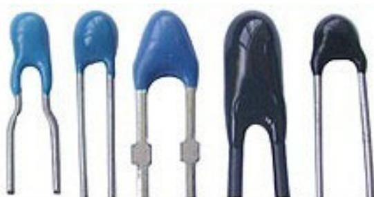
MF52 droplet temperature measuring type NTC thermistor is the negative temperature coefficient thermistor encapsulated by epoxy resin, and is featured by small size, high precision, quick response and stable performance.
